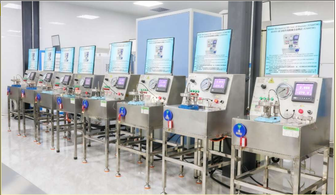
Set of diastats mechanical life test automatic equipment. Each equipment is equipped with a data recorder of testing parameters and number of cycles. (Ultimheat laboratory).
